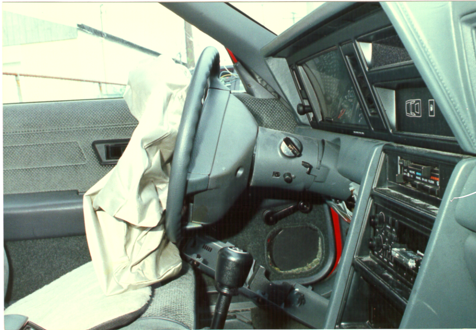
Steering Wheel Deformation And Column Compression That Resulted From Occupant Loading.
